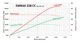
Fig. 3. External characteristics of the EMRAX 228 motor [13]
