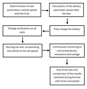
Fig. 18. Battery test flowchart
