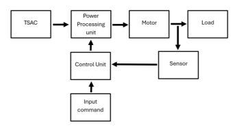
Fig. 2. Block diagram of a tractive system
