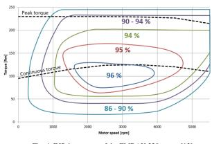
Fig. 4. Efficiency map of the EMRAX 228 motor [13]
