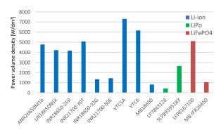
Fig. 7. Power volume density of selected cells
