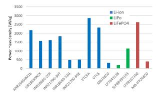
Fig. 5. Power mass density of selected cells
