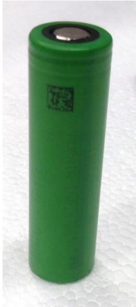
Fig. 11. VTC6 cell used
