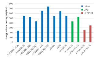
Fig. 8. Energy volume density of selected cells
