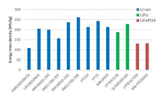
Fig. 6. Energy mass density of selected cells
